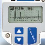
WaveForm display allows engineer/technician to view measurements in real-time
